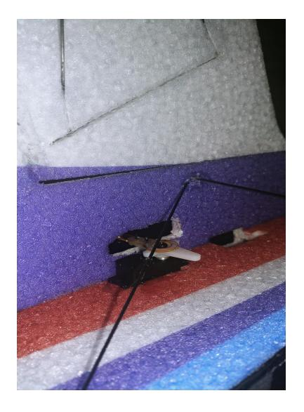
Shown above is the glued in elevator servo. For the elevator, use the middle servo slot that is on the side of the fuselage. The arms used for the elevator and rudder servos are the singles. For both the elevator and rudder servos, face the output shaft towards the rear.
