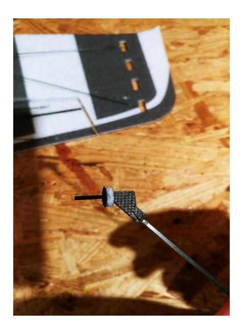
Shown above is one of the carbon fiber landing gear legs that come pre-glued to the axle. The larger of the two EPP foam circular collars will slide on first.
