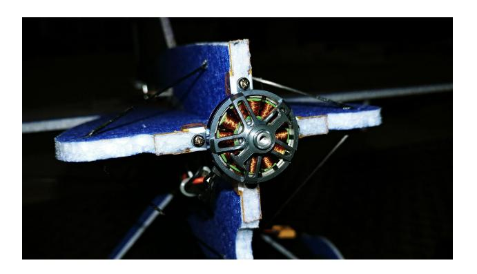
Shown above is the motor mounted to the provided motor mount.
