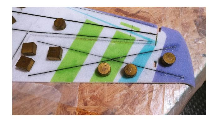
As shown above, the aileron bracing is done using flat carbon fiber glued into the slots creating durability for the aileron. Please see the carbon fiber diagram for your airframe to determine which size carbon strips are to be used.
