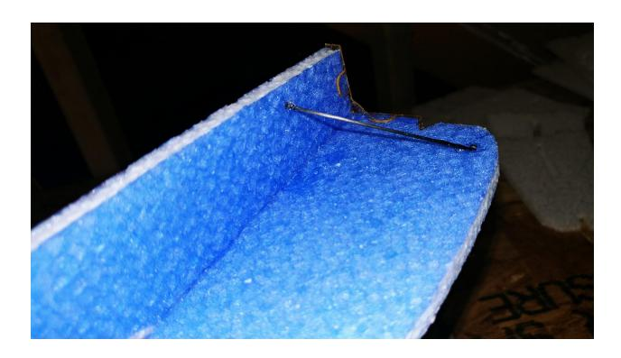
The final piece used for carbon fiber bracing will be the rod used at the front of the airframe. Make sure that the fuselage is straight while these pieces are setting.
