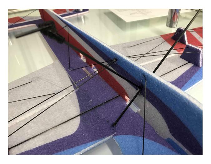
Above is the other side of the fuselage carbon fiber arrangement.
