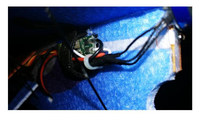
Shown above is the ESC mounted using the velcro strap and a supplied zip tie is used to tie the ESC wires together.
