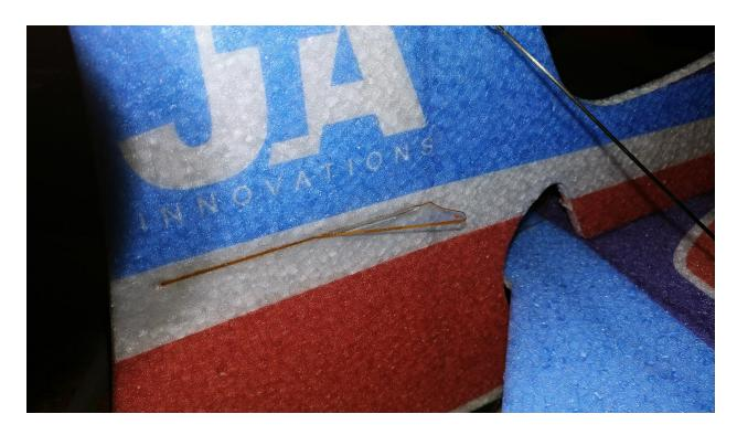
You can now locate the final long control horn and glue it into the slot on the side of the rudder. This will be used for the rudder linkage that will be constructed in the same way as the one used for the elevator. Once again, the length for that linkage is 365mm. The guides for the rudder linkage will be glued into the top of the vertical fuselage.
