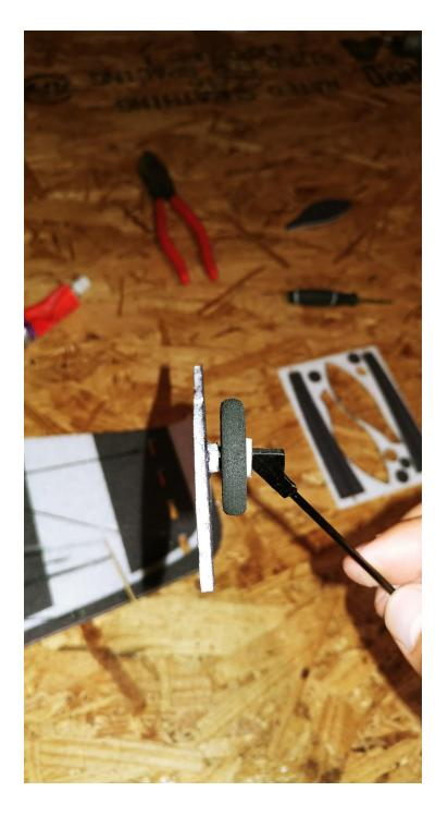
Lastly, locate one of the wheel pants. You can place a bit of adhesive on the last foam collar before sliding the wheel pant on to the axle. If desired, you can place some adhesive on the outside of the wheel pant where the carbon fiber axle ends.
