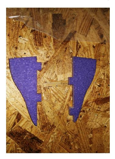
If desired, locate the side force generators that will be glued into the counterbalances of the ailerons. \*Some airframes may require the SFGs to be glued into different locations along the wing.\*
