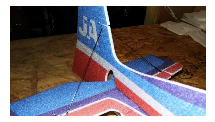
Shown above is the carbon rod that will go on each side of the fuselage. It will be used to strengthen the horizontal stab and vertical stab.
