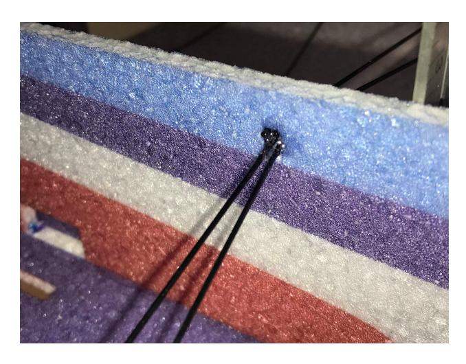
Shown above is the wing bracing glued into the bottom part of the fuselage.
