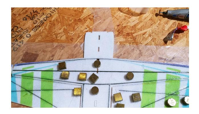
Wing bracing shown above. The center wing spar is the supplied carbon fiber square stock.
