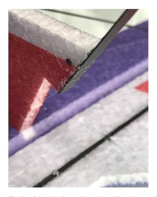
Glue the tailpiece into place as shown above while making sure that it is on the same angle of the bottom of the fuselage to ensure that the airframe will sit level.
