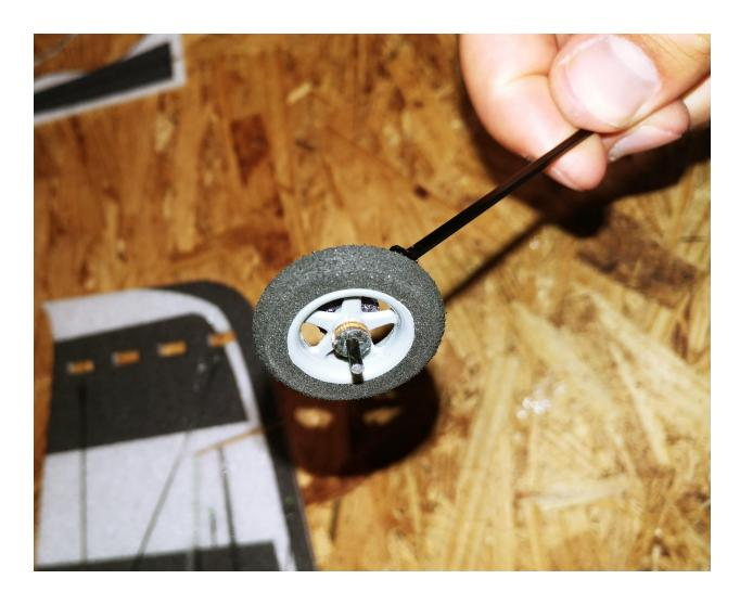
Now locate the plywood/carbon fiber laminated collar to slide up next to the plastic wheel. Once again, do not apply glue yet as the tire will need to spin as freely as possible around the axle.
