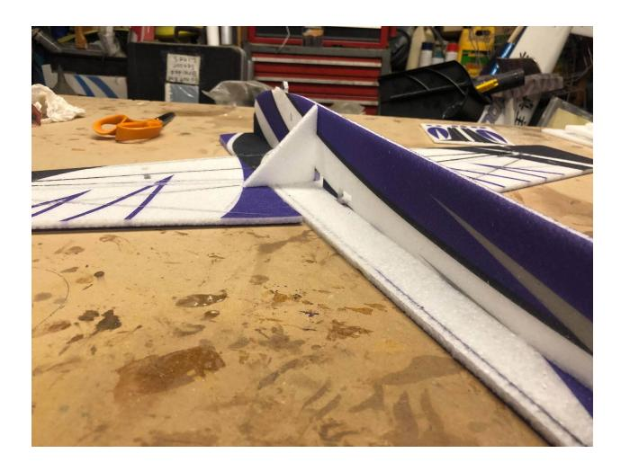
The provided EPP square may be useful during this process of gluing the bottom fuselage piece.
