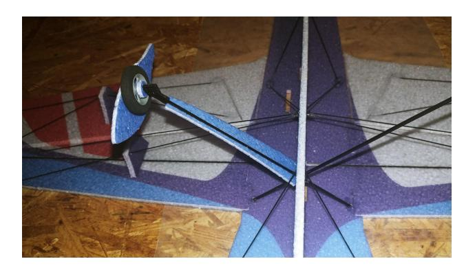
Locate the EPP landing gear cover that will be placed over the carbon fiber landing gear leg. Test fit this piece, then glue it on over the carbon fiber using the pre-cut slot.
