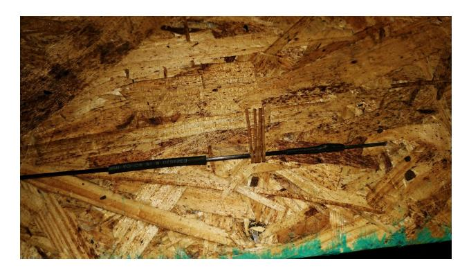
Shown above is the elevator linkage. Notice how the 4 guides are slid over the linkage and the heatshrink is cut and slid on before the Z bend is glued. The rudder linkage will be done the same way later on. You will be able to tell where the guides will need to be glued in based on the slots in the fuselage.
