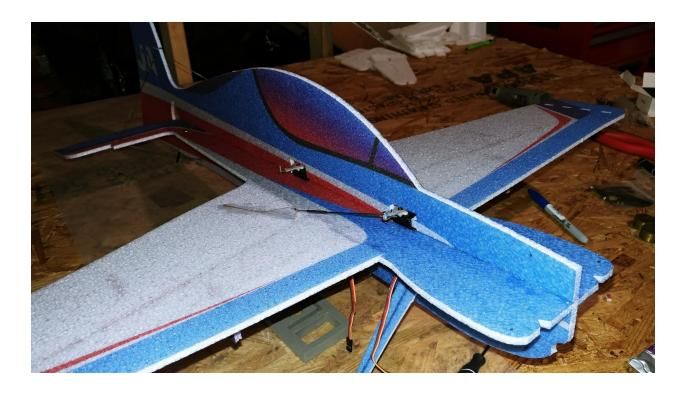
Once the aileron and elevator linkages are set up, use the same process as glueing the bottom of the fuse to glue the top of the fuselage into place. Once again, it is important to keep this as straight as possible.
