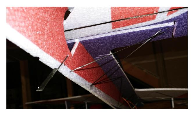
Now that the top of the fuselage is glued in, you can glue the other rear carbon fiber rods to help strengthen the tail as shown above. They will be mounted from the bottom of the horizontal tail to the rear of the bottom vertical fuselage. Make sure they are glued in a location that allows for full down elevator throw.
