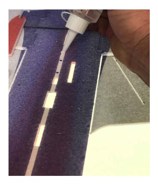
Using the marks that you just made, place your glue along the fuselage.
