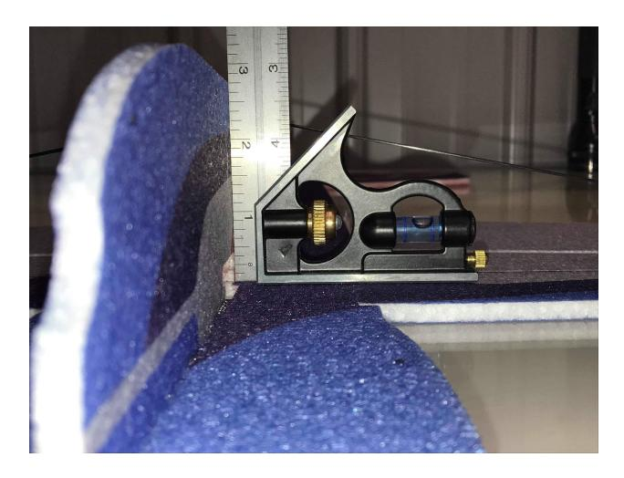
It is extremely important to make sure that the bottom vertical part of the fuselage stays 90 degrees to the horizontal fuselage while the glue is setting. This can have a huge effect on the flying characteristics.
