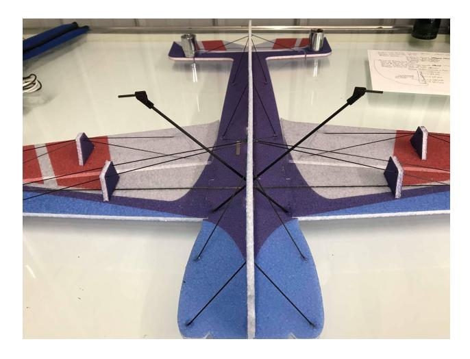
Shown above are both landing gear legs in place. You will find the slots cut in the side of the bottom of the fuselage to slide each landing gear leg into. Make sure that the bottom of each leg is placed to where the airplane will sit level on the ground. Also shown are the first two carbon braces on the front of each side of the bottom of the fuselage.
