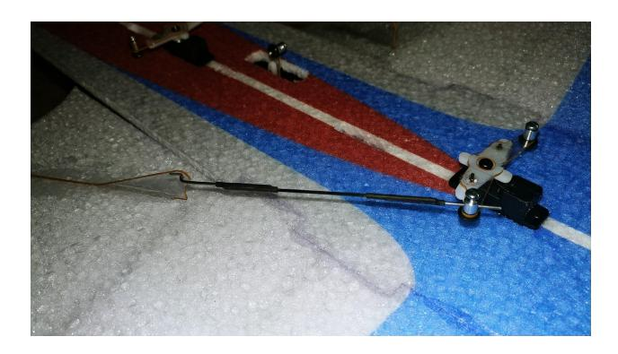
Shown above is the entire aileron linkage assembly for one aileron. Notice the heat shrink over each glued end, as well as the straight end clamped into the mini EZ connector on the servo arm.
