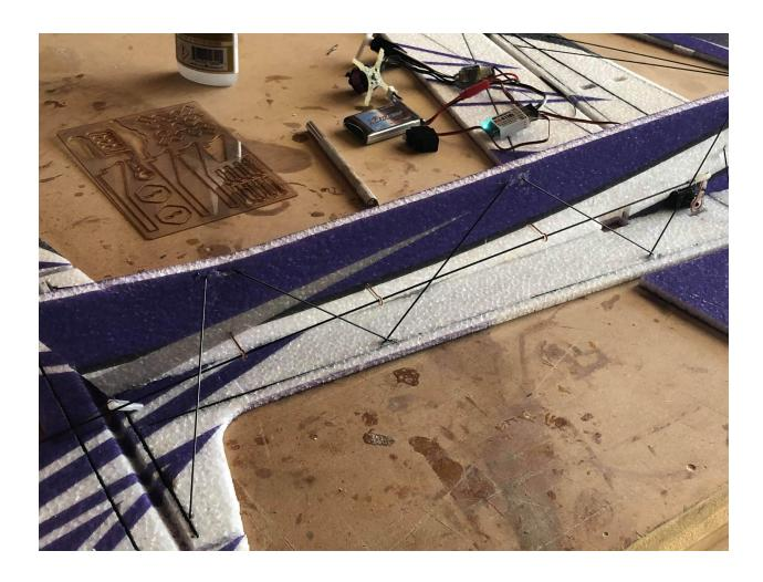
Shown above is the bottom fuse bracing for the rear of the fuselage. Lengths found in diagram.
