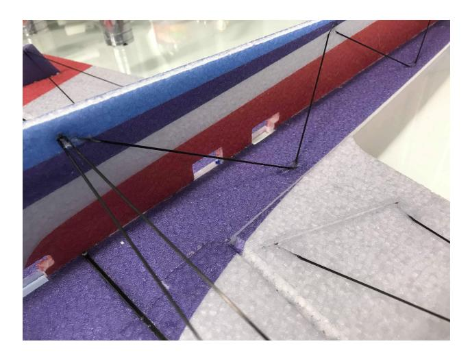
Shown above is the rest of the bottom fuselage bracing up to the wing bracing. You should be able to notice the dots marked to help guide where each rod will be placed. Lengths found in diagram.
