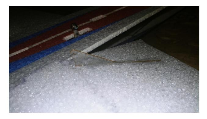
Shown above is one of the aileron horns in place on the top of the aileron.
